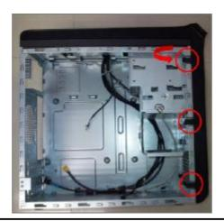
**2.2** Disconnect the cable housing then you can remove front bezel.
